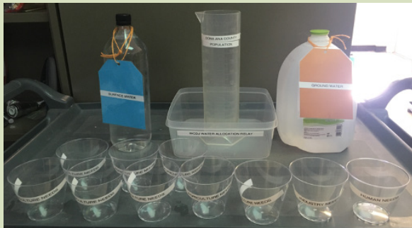
Figure 1. Year of Plenty setup, including 10 small cups, one 1000-mL graduated cylinder, a one-gallon bottle filled with water, a 1-L bottle filled with water, and an overflow container
