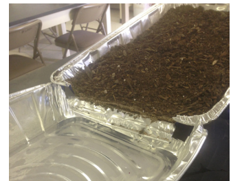
Figure 6. Attachment of soil pan to catch pan
