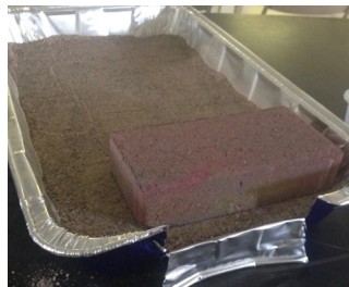
Figure 5. Lower layer of play sand in the soil pan, tamped down so that sand is flush with opening
