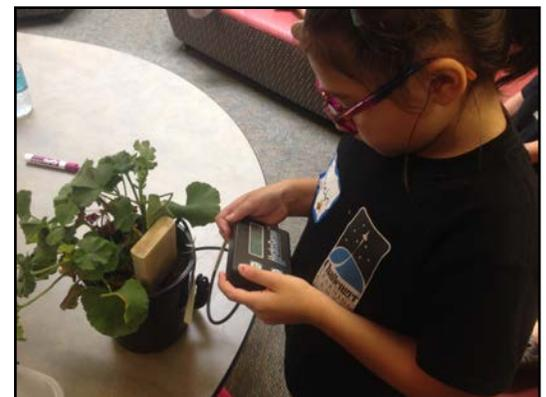
*Micro Explorers use a soil moisture probe to monitor water availability in the soil.*
